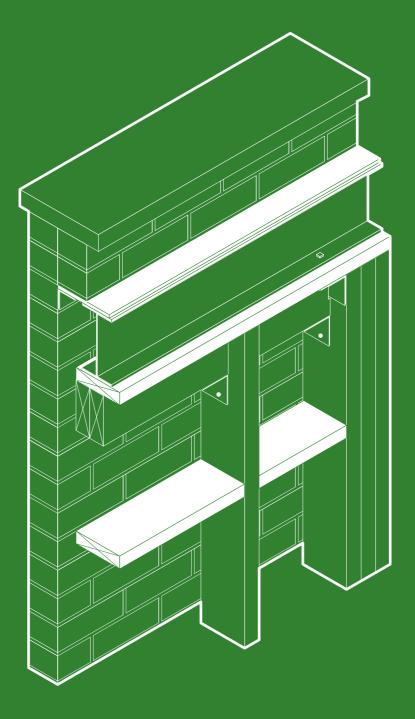
310.01 - BOW, LONDON - PARAPET SUPPORT STUDY - ISOMETRIC NOT TO SCALE
